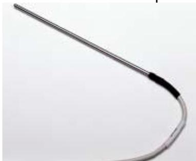
Plug this sensor into the Port labeled: I/O 1. The arrow on the plug of the temperature probe should face down. As you face the Nova, it is the port on the right. If the probe is not plugged into port 1, the NOVA5000 will not recognize it.
